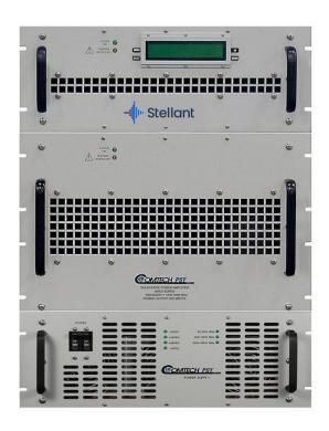
quieting (blanking) feature is provided and noise power output is reduced to a level of -150dbm/Hz in less then 50 Microseconds. All amplifiers include self contained rugged power supplies; primary AC input is 208VAC (3) phase.
